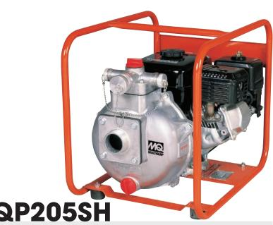
2" Suction • 1" and 1.5" Discharge • 106 GPM Flow 230' Head • 100 PSI • Honda GX160, 4.8 HP
