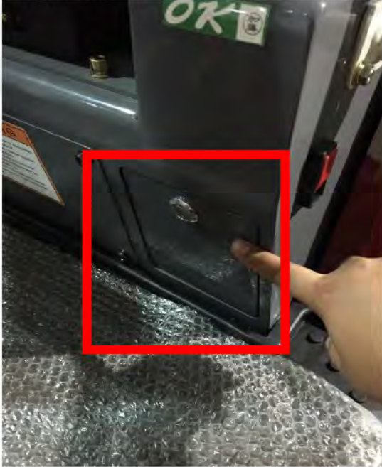
TB230 TB240 TB260 Uninstalled Fuse Example
