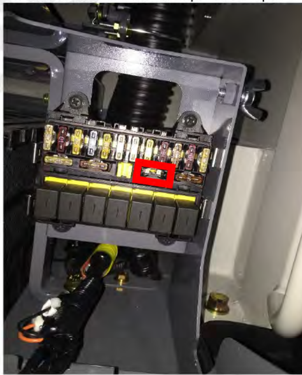
TB290 Uninstalled Fuse Example Cover Open
