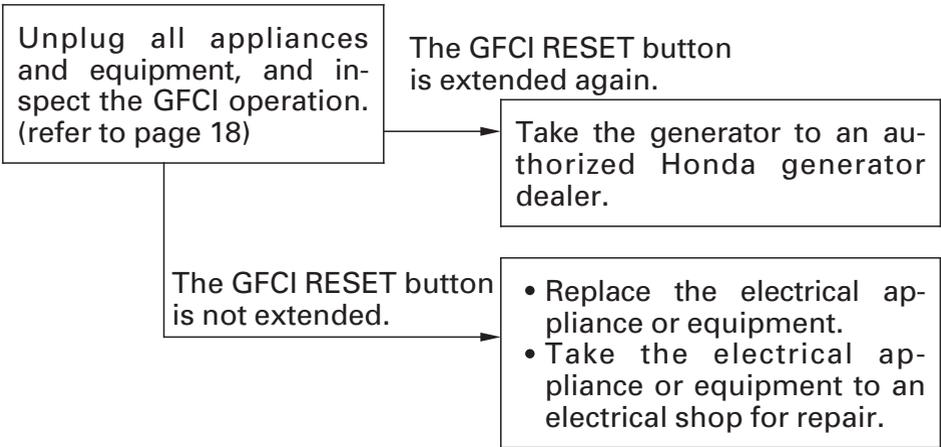
〈When the GFCI RESET button is not extended〉
