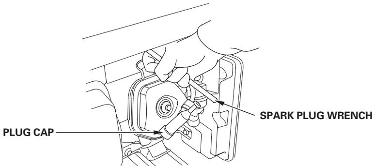
4. Visually inspect the spark plug. Discard it if the insulator is cracked, chipped or fouled.
