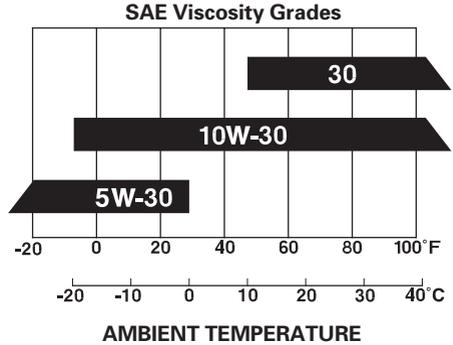
SAE 10W-30 is recommended for general, all-temperature use. Other viscosities shown in the chart may be used when the average temperature in your area is within the indicated range.
