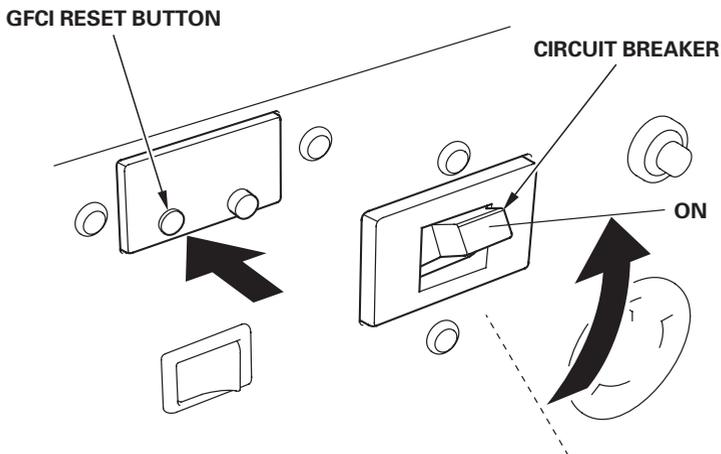
During generator use, if the GFCI RESET button extends and the circuit breaker trips, this usually indicates a faulty power tool, appliance, or cord.
