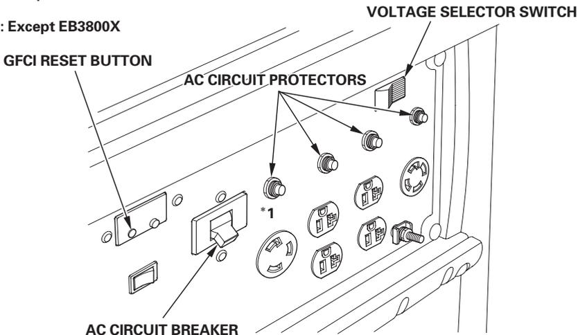
Do not exceed the current limit specified for any one receptacle. If an overloaded circuit causes the AC circuit breaker or circuit protector to switch OFF, reduce the electrical load on the circuit, wait a few minutes and then reset the circuit breaker or circuit protector.
