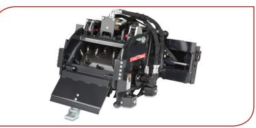
The Bradco Cold Planer, by Paladin, is an effective tool for small milling jobs, as well as asphalt and concrete pothole and frost heave repair, curb cutting, pavement texturing and removal of traffic lane stripes and roadway around manholes.
