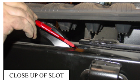
LOCATION OF SLOT FOR CHECKING TRACK TENSION
