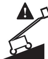
Light on indicates machine is not level. The tilt alarm will be sounding when this light is on. Move the machine to a firm level surface.
