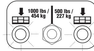
Two light blinking indicates that the capacity has not been selected.
