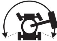
To drive, hold the drive enable switch to either side and slowly move the drive control handle off center.
