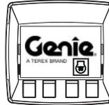
The LCD screen displays hour meter, voltage, oil pressure and coolant temperature. The screen also displays fault codes and other service information.
