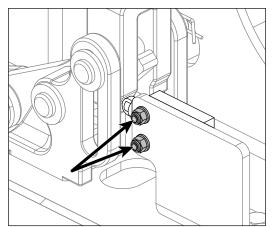
**4.** Remove the bolts and washers (x2) that secure the lock plates to the base. Set the hardware aside for later reinstallation.
