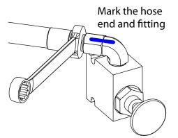
6. Referencing the chart below, use a second box wrench to tighten the nut the appropriate number of flats past the mark. Do NOT over tighten.
