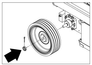
**7.** To limit rust bleed, it is recommended that a few drops of grease be applied to the two small tapped holes on the rear wheels.
