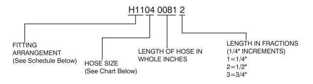
Using the number above as an example, H1104 0081 2, this hose requires a 37° JIC female swivel fitting on one end, and a medium length 90° JIC female swivel fitting for the other end. The hose must meet or exceed the S.A.E. 100R13 hose specification, and be a total of 81-1/2" long.
