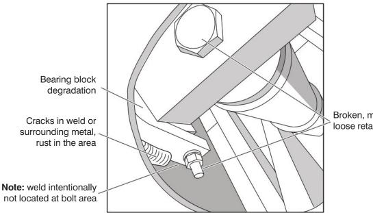
Broken, missing, or loose retainers or bolts
