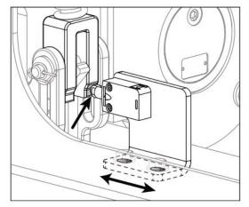
**3.** Tighten the hardware to secure the lock plates to the base. Make sure the limit switches do not move while you tighten the bolts and the plunger roller's retaining pins are fully visible.
