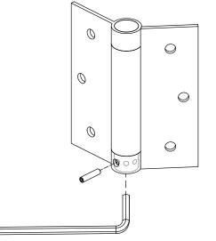
**4.** Adjust all the other spring hinges on the gate so they have the same tension.
