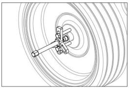
5. Use a hub puller to remove and discard the hub/ integrated hub wheel from the wheel motor or brake.
