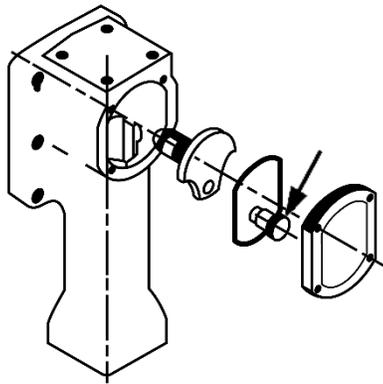
**Figure 7: Location of left-hand thread crank pin**
