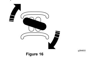
To turn left, rotate the traction control counterclockwise (Figure 17).
