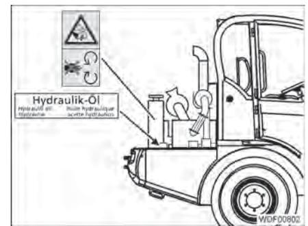
Fig. 4 Stickers located in the engine compartment (right)
