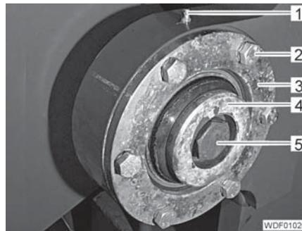
Fig. 297 Lower bearing attachment
