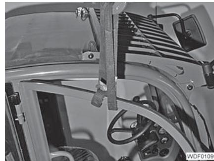
Fig. 382 Attaching lifting gear to the door
