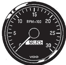
"SELECt", "PULSE" and "AdJUST" appear alternately every 3 seconds on the display. The function "PULSE" is required for Weidemann machines.
