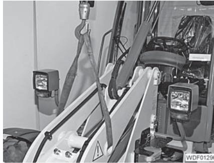
Fig. 312 Securing the load arm
