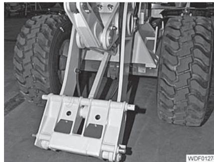
Fig. 191 Load arm in lowered position
