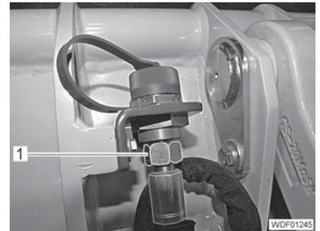
Fig. 230 Hydraulic connection
