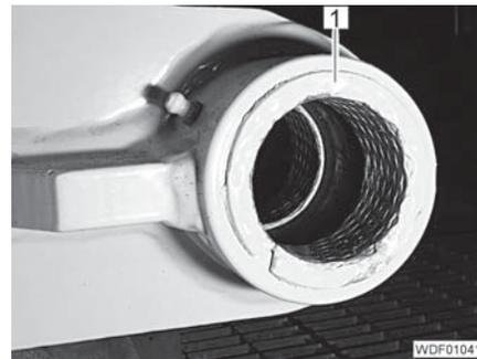
Fig. 321 Front bearing (right)
