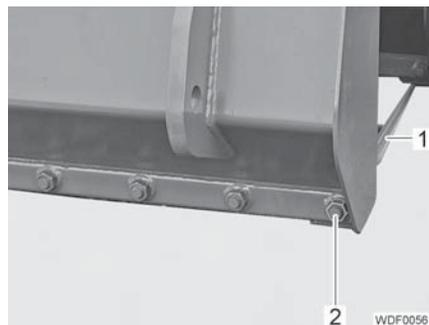
Fig. 471 Securing the prong
