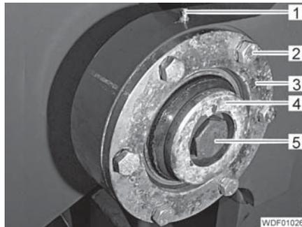
Fig. 287 Lower bearing attachment
