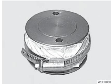
Fig. 106 Compression of the annular seal
