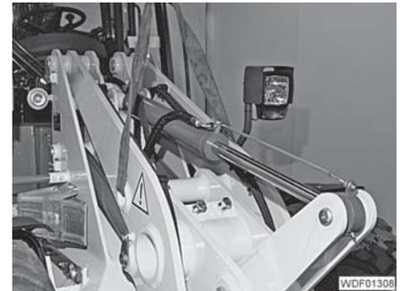
Fig. 323 Securing the load arm
