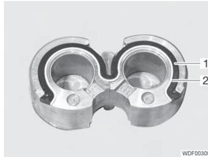
Fig. 160 Bearing seal
