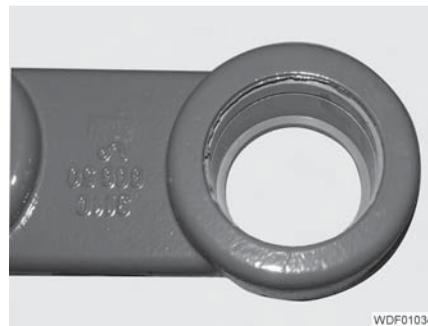
Fig. 302 Underside of the self-aligning bearing
