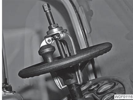
Fig. 397 Pulling off the steering wheel
