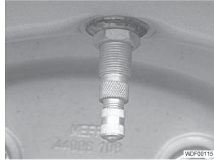
Fig. 40 Water filling valve
