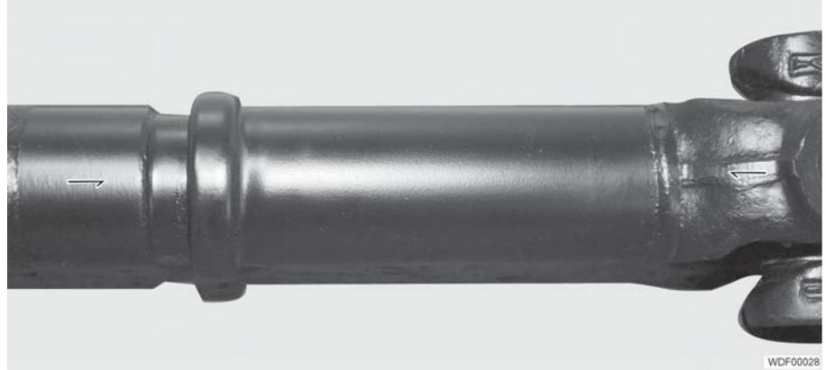
Fig. 231 Markings on the drive shaft
