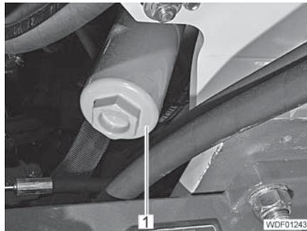
Fig. 227 Filter housing of the pressure filter
