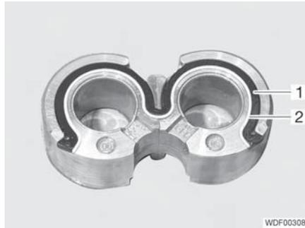
Fig. 150 Bearing seal
