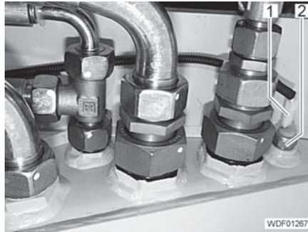
Fig. 433 Connections on the hydraulic fluid tank
