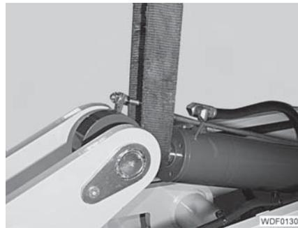
Fig. 316 Attaching the tipping cylinder
