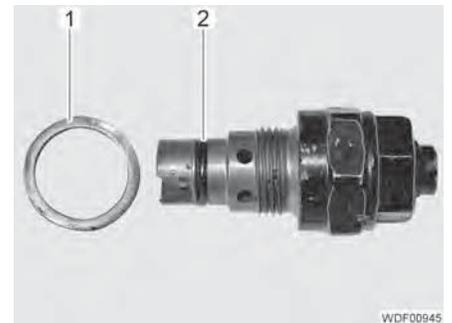
Fig. 174 Pressure control valve
