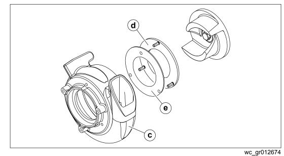
4. Check clearance between the impeller and the insert by slowly pulling the starter rope to turn the impeller. If starter rope is difficult to pull, or rubbing is heard from inside pump, the impeller and insert are too close to each other. Remove a shim (e) from behind the insert and check again for rubbing. Continue removing shims until the impeller turns easily.
