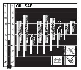
Choose the recommended viscosity based on the type of start (recoil, crankhandle or electric) and on the engine temperature at which the engine will be operated.
