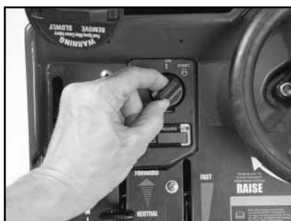
(G) Start engine by rotating Ignition Switch to the right.
