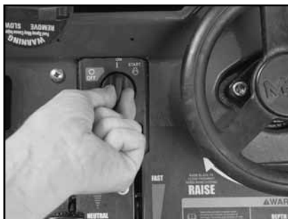
(A) Place Engine Master Switch in the OFF position.
