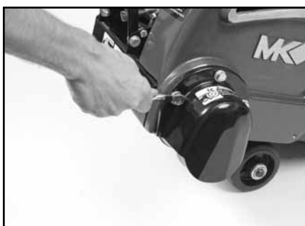
(E) Locate the Blade Shaft Cover Retaining Bolts.
