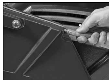
(I) Install the Cooling Transfer Hose to the Blade Guard.
