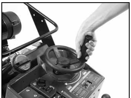
(K) When the cut is complete, raise the Blade completely out of the cut by turning Depth Control Wheel counter-clockwise.
