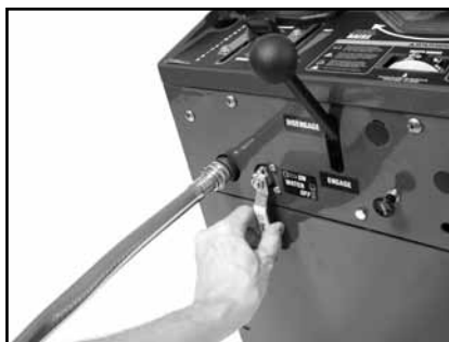
(L) Close Cooling Supply Valve.
