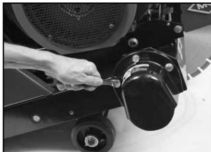
(J) Install the Blade Shaft Cover.
