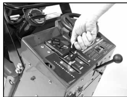
(F) Push Engine Throttle Handle up half-way.
