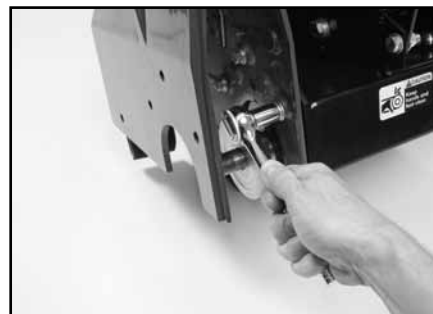
(C) Locate the four Blade Guard Retaining Bolts.
