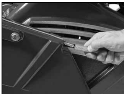
(B) Remove the Cooling Transfer Hose from the Blade Guard by pressing the quick release.
