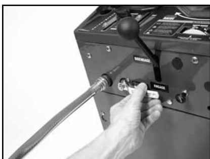
(H) For Wet Cutting, open Cooling Supply Valve. Verify proper cooling flow and adjust the water flow on the Blade to a desired amount.
