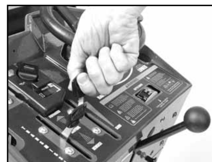
(I) Move the throttle all the way for- ward to "Fast" position.
