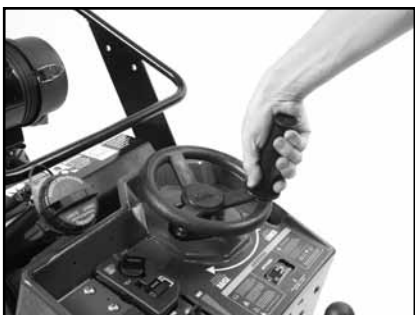
(J) Slowly lower the Blade until the desired level is reached and begin the cut.
