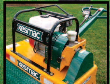
Optional power unit protection package with lift eye and dead man's handle.
