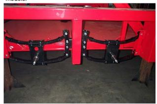
Figure 4-9. Dual, Quadra Spring Suspension
