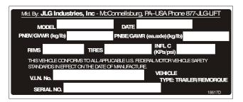
Figure 2-2. Vehicle Identification Plate
