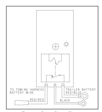
Figure 3-1. Battery Charger Diagram
