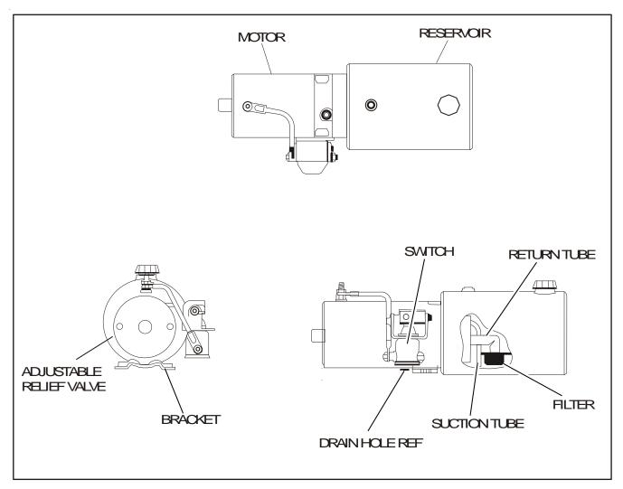
Figure 4-4. 12 Volt Motor/Pump Parts
