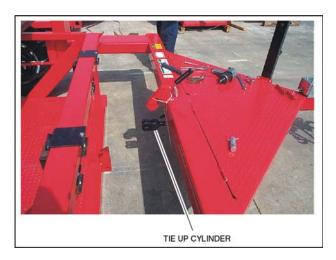
8. Using the "up/down" control, collapse the cylinder just enough to free it from the deck. Tie up the cylinder so that it will not fall to the ground when lifting the frame. Do not collapse the cylinder any more than necessary to be free from the deck since you will need to manually extend the cylinder when reassembling.
