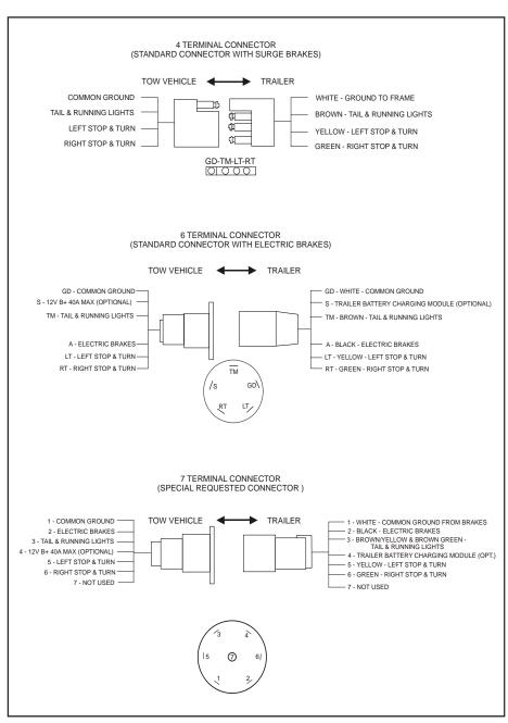
Figure 4-7. Trailer Connections
