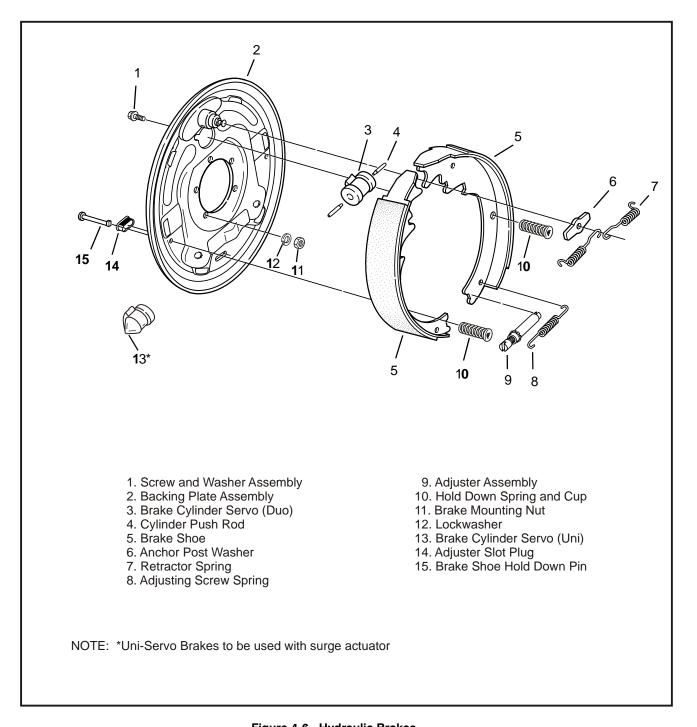
Figure 4-6. Hydraulic Brakes
