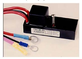
Disconnects trailer battery from vehicle's charge wire when not charging, (engine is not running) preventing two dead batteries.
