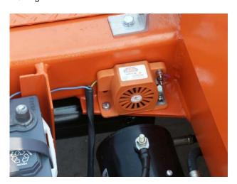
The alarm should sound automatically when the deck control lever is moved to the "down" position
