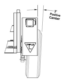
Figure 4-11. Suspension Camber Setting (Fixed)
