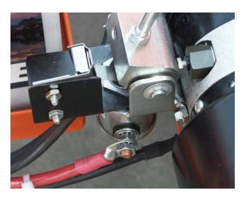
Switch is mounted directly to the starter solenoid located under the deck control lever. The switch is activated when the deck control lever is moved to the "down" position.
