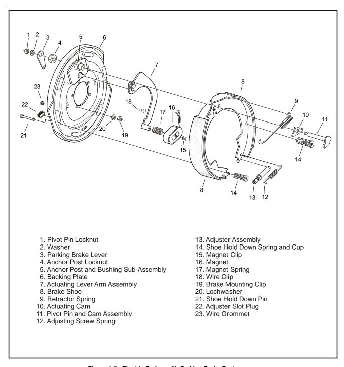
Figure 4-5. Electric Brakes with Parking Brake Feature
