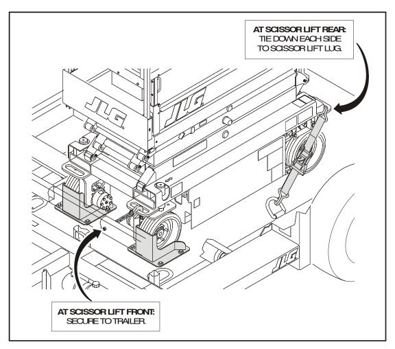
Figure 3-2. Tie Down Attach Points
