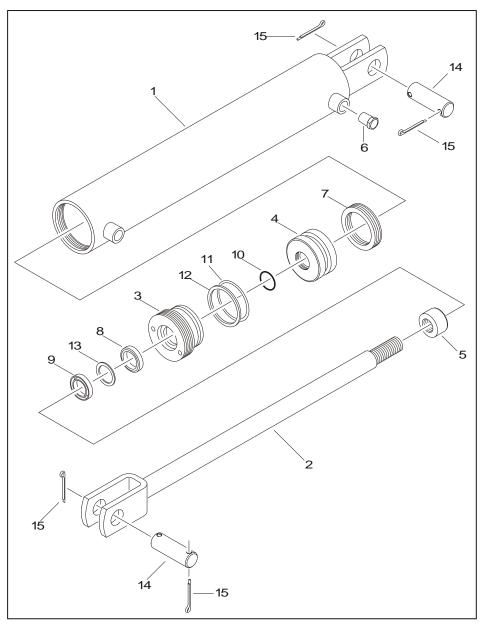
Figure 4-2. Hydraulic Cylinder
