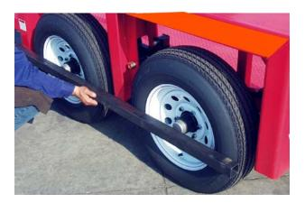
To check wheel alignment, position a straight edge at the center line of the wheels and see that all sidewalls are in alignment. Because of movement of tandem axles when turning, be sure trailer has been pulled in a straight line before checking. If correction is needed, loosen the 8 spring pad bolts (4 at top and 4 at the bottom spring) and then reposition wheel. Once corrected, retighten all bolts. Torque to specified ft. lbs. (Refer to Table 4-5, Wheel Torque Chart).
