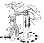
Remove any undergrowth from the base of the tree and check the area for obstacles (stones, branches, holes, etc.) so that you have a clear path of retreat when the tree
