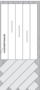
Plank and Strip Floors - sand in the direction the boards are laid, with the wood grain.
