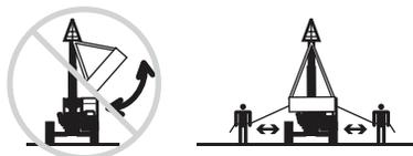
Do not permit the load to swing freely. Always properly tether loads to restrict movement. Driving across grades, sudden starts, stops, and turns can cause the load to swing and create a hazard if not externally stabilized.
