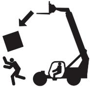
Keep people, equipment and material out of the work area. Do not operate the machine while people are under or near an elevated boom, whether it is loaded or unloaded.
