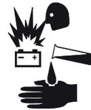
Refuel the machine and charge the battery only in an open, well-ventilated area away from sparks, flames and lighted tobacco.
