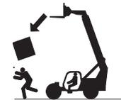
Do not raise a load unless the load is properly positioned or secured on the forks or approved attachment.
