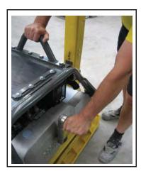
5. Grasp handle grip with one hand, with the other hand support the protective cage.
