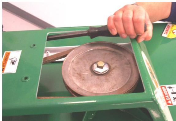
Adjusting Blade Drive Belt Tension
