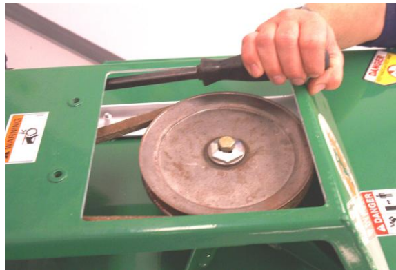
Adjusting Blade Drive Belt Tension
