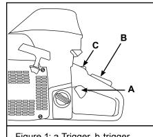
Figure 1: a-Trigger, b-trigger interlock, c-throttle lock
