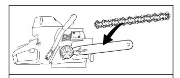
STEP 4 Mount the diamond chain on the guide bar starting at the drive sprocket and continue over the guide bar nose.
