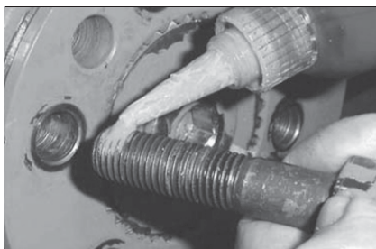
Fig. 72: Loctite 242 on securing ring screws
