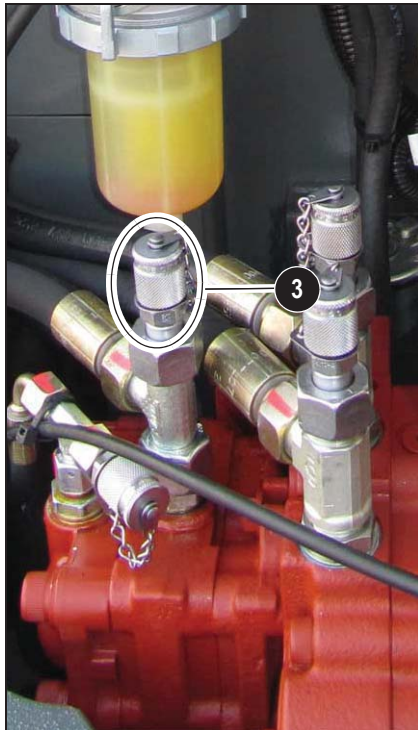
Fig. 44: Measuring port P3
