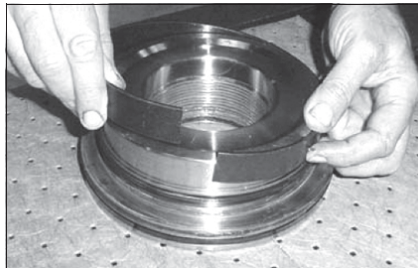
Fig. 24: Removing the seals and bearings
