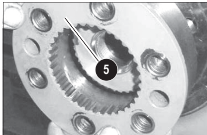
Fig. 59: Installing the securing ring
