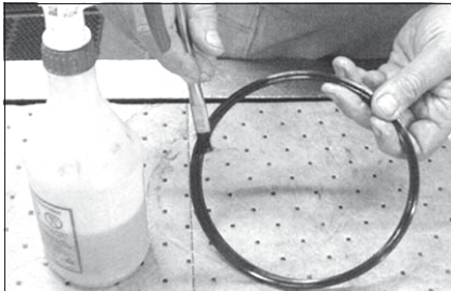
Fig. 32: Coat the seals and surfaces with oil
