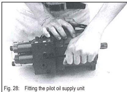
Fig. 28: Fitting the pilot oil supply unit
