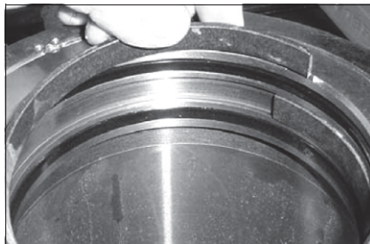
Fig. 40: Fitting the wear indicators
