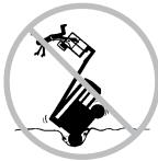
Use extreme care and slow speeds while driving the machine in the stowed position across uneven terrain, debris, unstable or slippery surfaces and near holes and drop-offs. Do not drive the machine on or near uneven terrain, unstable surfaces or other hazardous conditions with the boom raised or extended.
