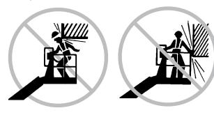
Be aware of crushing hazards when grasping the platform guard rail.
