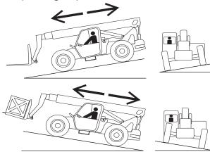
DO NOT use frame leveling when boom is elevated. Only use frame leveling when boom is retracted and in lowered position.
