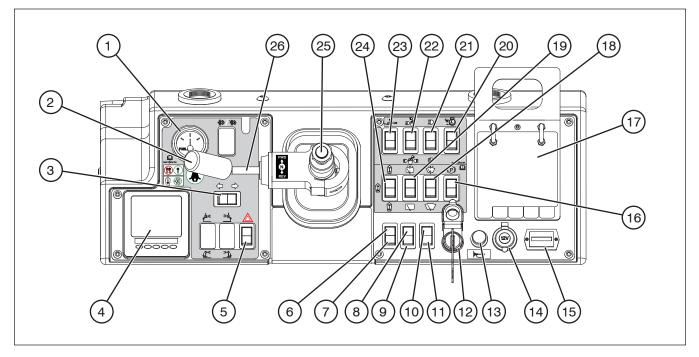
When in "O" OFF position, it turns the engine off and key can be removed. When in "I" ON position, it provides power to ignition and auxiliary circuits. When in "II" START position, it starts the engine; when released, key returns to "I" ON position.
