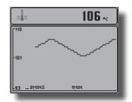
Figure 2-10 Example of Graphic Display Showing Coolant Temperature
