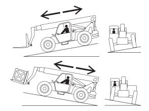
Figure 2-19. Driving on a Slope
