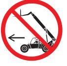
**DO NOT** operate on surfaces not capable of holding the weight of the telehandler; including the rated load (e.g., covers, drains, and trenches).
