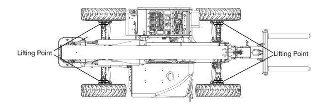
Figure 2-36 Center of gravity and lifting points
