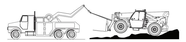
Fig 2-37 Towing the telehandler from front tie-down points
