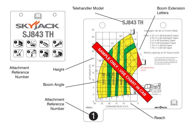
Fig 2-23 Sample Capacity Chart
