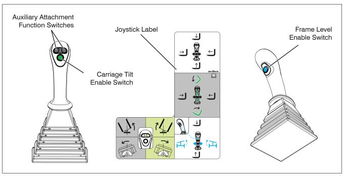
Test Boom and Attachment Functions
