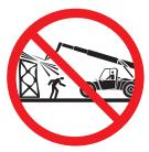
• **DO NOT** elevate the boom while the telehandler is on a truck, forklift or other device or vehicle.
