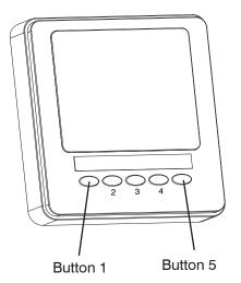
Figure 2-3 Engine Data Display Module
