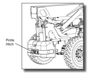
Figure 2-39 Pintle Hitch at rear of telehandler
