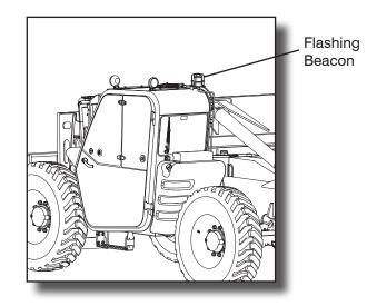
Figure 2-15 Flashing Beacon
