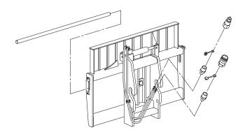
Figure 2-30 Side Tilt Carriage
