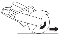
Never move the machine when the cutting equipment is rotating. Gyroscopic forces can obstruct the intended movement.
